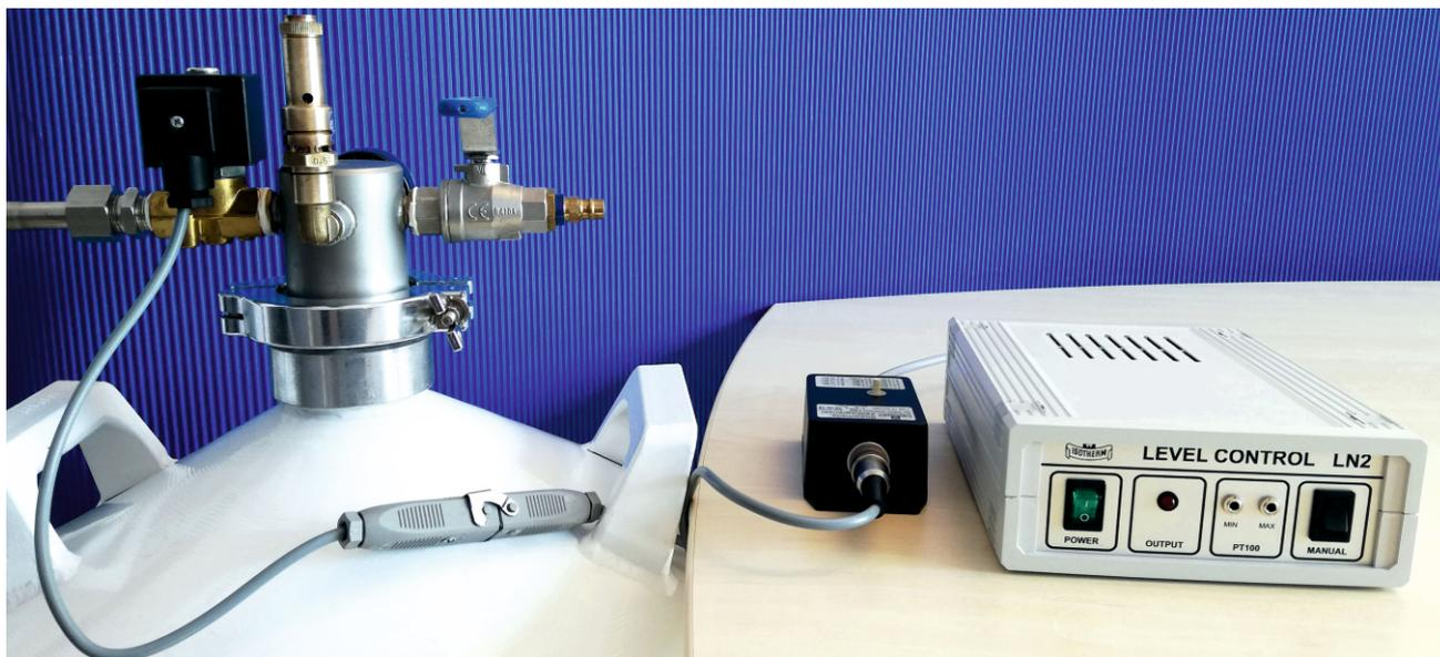
Automatic "Level Control LN2" type LN2 level regulation devices by KGW-ISOTHERM are used in many cryotechnical applications, such as the shrinking of shafts and bushes in LN2, deep-freezing of components or biological samples, use of LN2 as a coolant for cold traps, calibration of sensors in LN2, etc.
